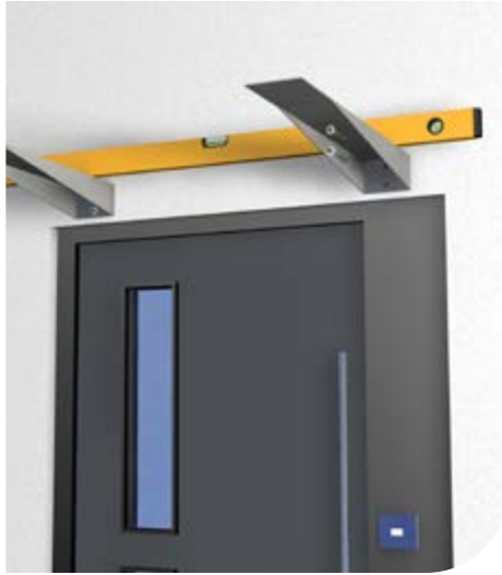
3. Level the wall bracket with a spirit level and check the position of the second wall bracket. Fit the second bracket into position. Double check level after fixing, and adjust or pack as required.
