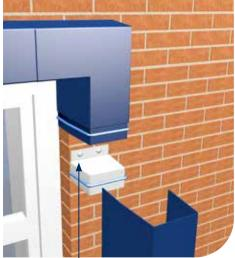
Always install vertical brackets with fixing holes on top to ensure maximum strength of the cantilever design.
